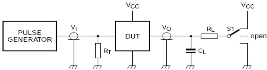
**Fig 8. Load circuitry for measuring switching times**
