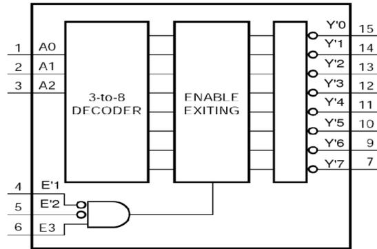
**Fig2. Functional diagram**
